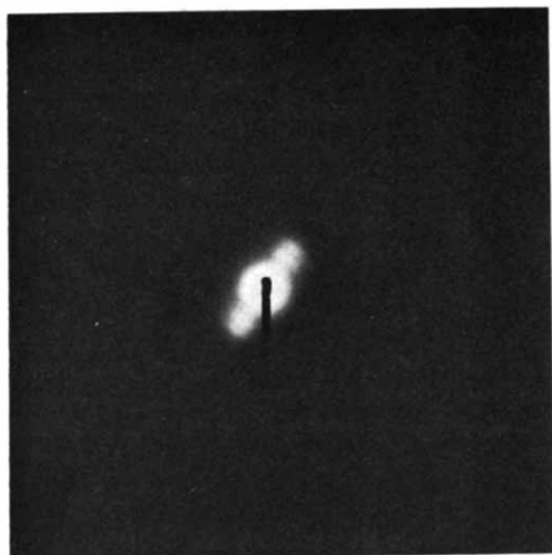
Fig. 3. Diffraction pattern of an agglutinated sheep red blood cell membrane pellet prepared with 10^{-4} \text{ M HgCl}_2 . The meridional reflections at (60 \text{ \AA})^{-1} and (45 \text{ \AA})^{-1} are shown. (Specimen-to-film distance 108.7 mm. Print magnification 1.5 \times .)
